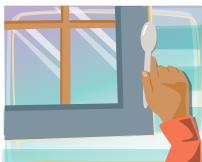
Once you have applied the caulk, it takes time for it to dry, or cure. Curing time is described two ways. The tack-free time tells you how quickly the fresh caulk's outer surface will dry—or skin over. The total cure time indicates the time required for the caulk to become completely stable—or reach the point where no further drying or shrinking will occur.
